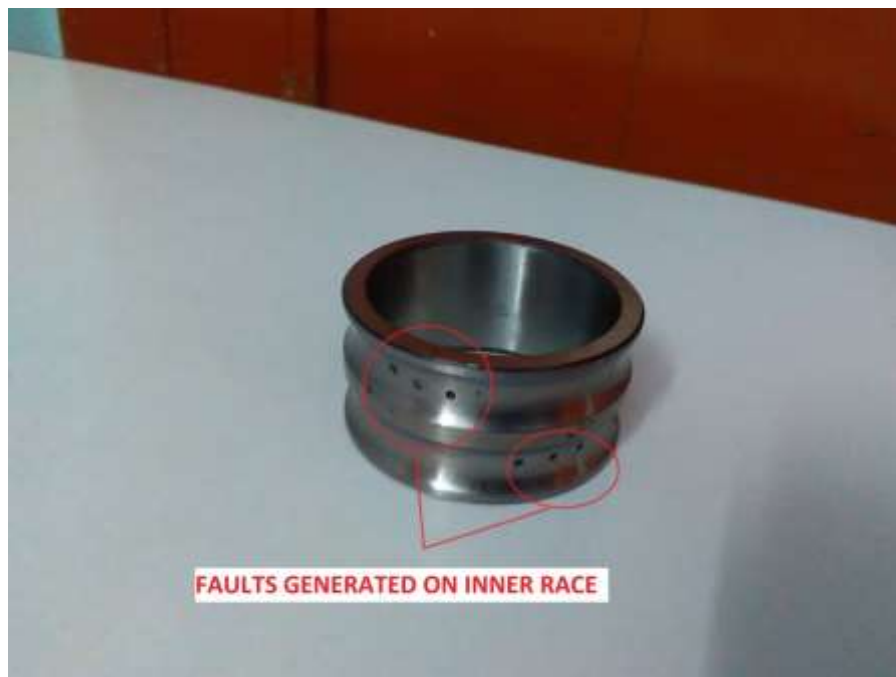
Figure 2. Inner race of bearing possessing inner race defect
