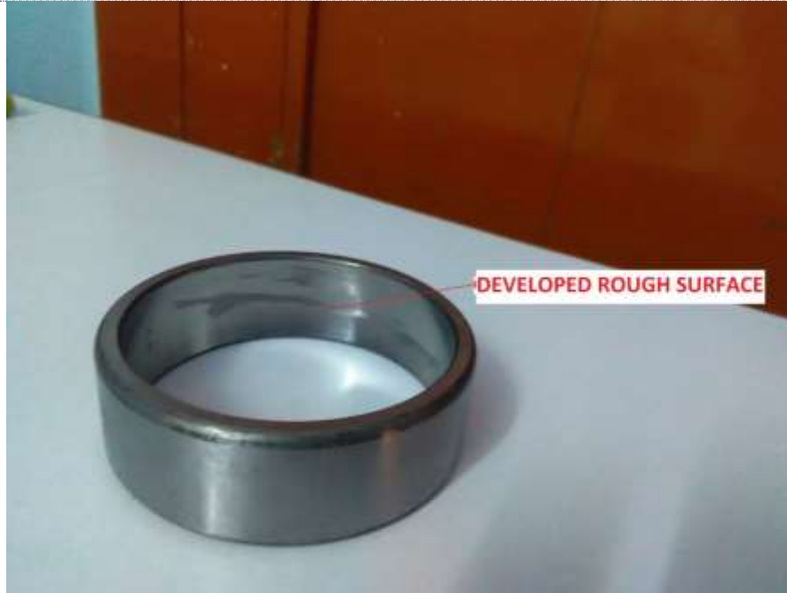
Figure 3. Rough surface of bearing possessing rough surface defect
