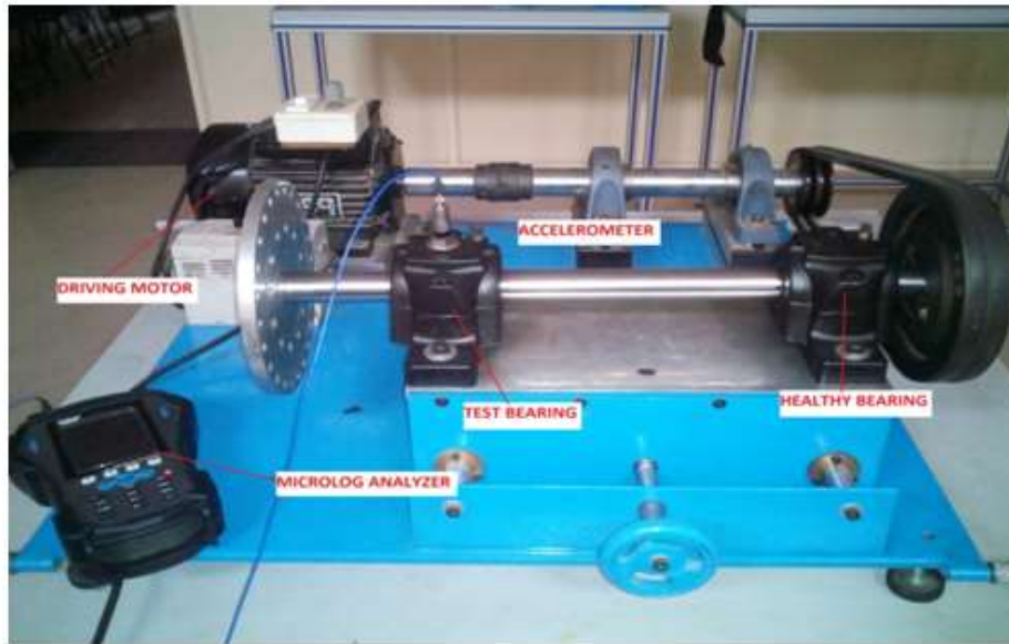
Figure 1. Fault Simulator testing rig
